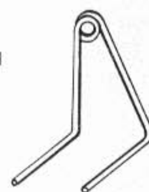
EXTERNAL HORN Sew and epoxy to elevator.
