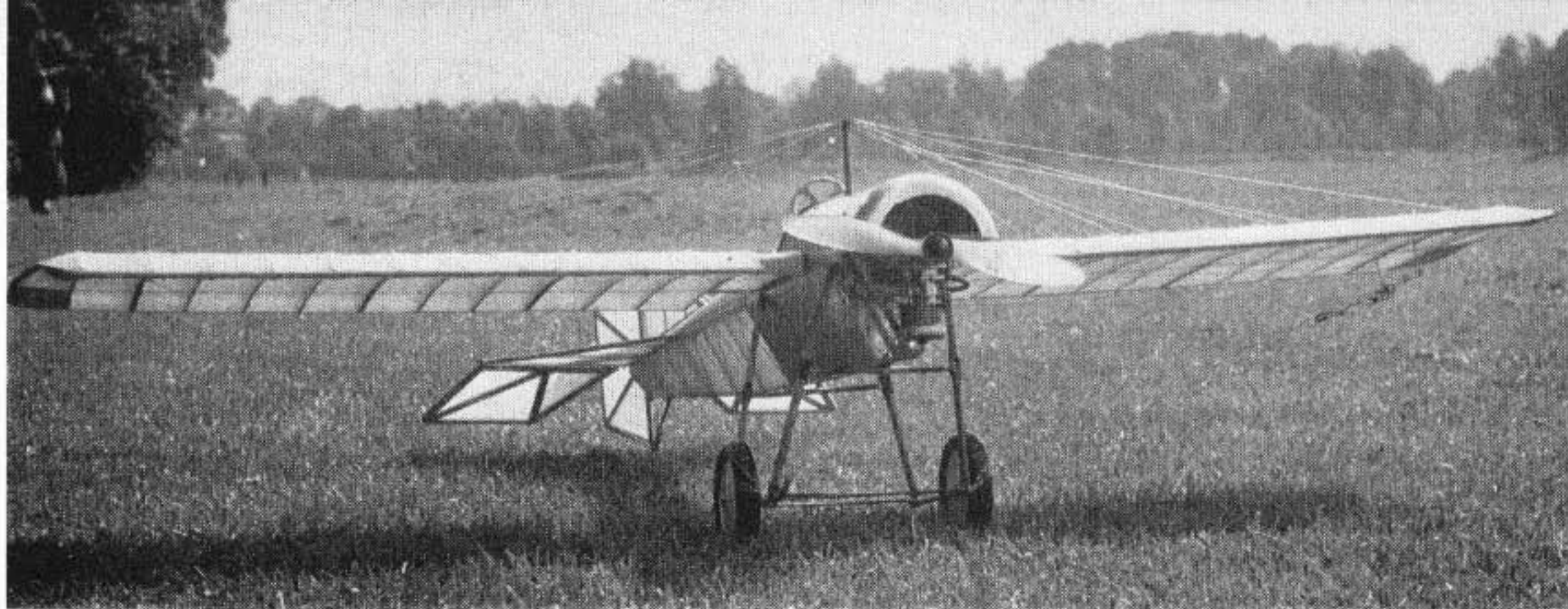
A nice slow, realistic flier is this Blackburn 1912 Monoplane for Fox 25 R/C power – throttle control makes it all the more interesting in flight. The Aero Modeller free flight plan (FSP 567, price £1.15) could be adapted with hardwood spars, no wing incidence and stronger engine bearers.
