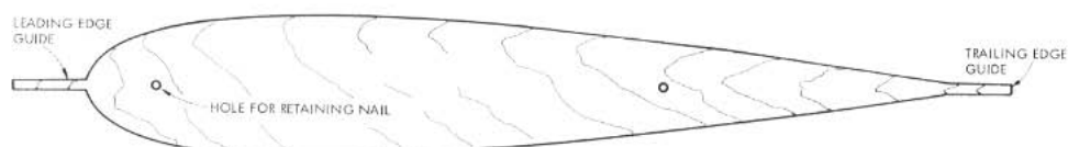
Figure 2 — Typical wing template. Use nails to fix to either end of foam blank. When cutting the foam, place the blank between wooden stops screwed to the workbench and then place a book or similar large heavy object on top of the blank to keep it firmly in place. You need both hands to operate the hot wire cutter.
