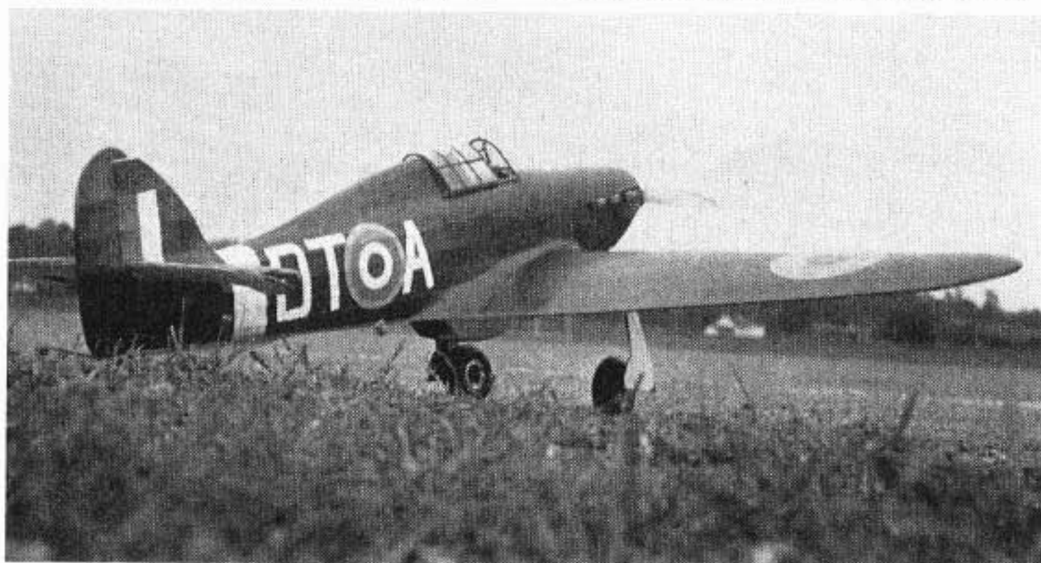
Hawker Hurricane converted from the AeroModeller free-flight by Richard Cooke of the Sudbury club. Power is provided by a PAW 19 diesel. This is one of the few WWII fighter aircraft suitable for this 'stand-off scale' approach to modelling.
