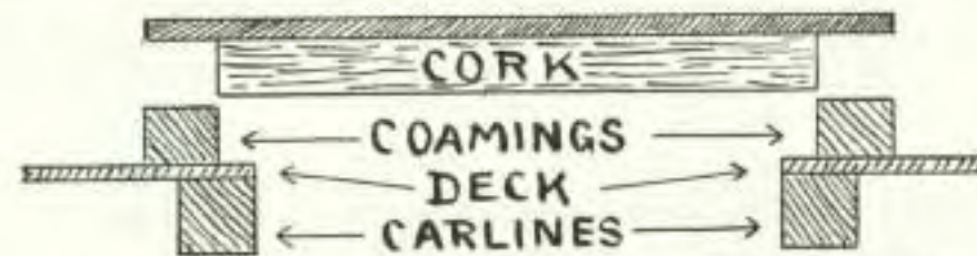
Fig. 18—HOW TO MAKE A WATERTIGHT HATCH
