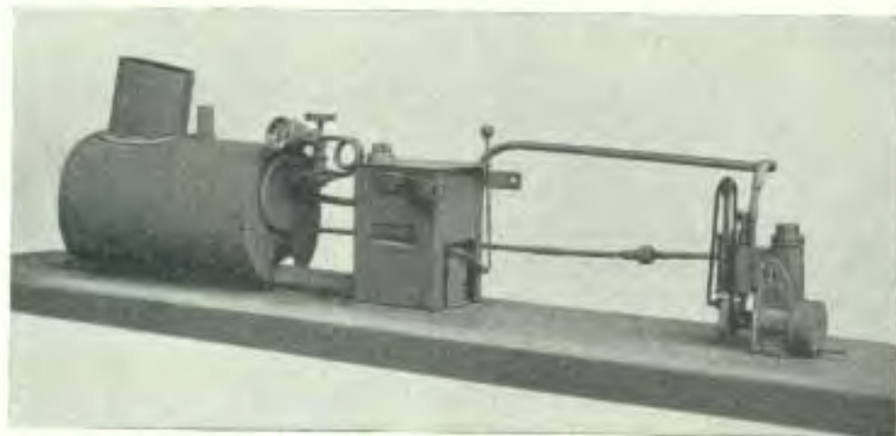
THE BASSETT-LOWKE No. 94 ENGINE. Complete with Boiler and Lamp.
