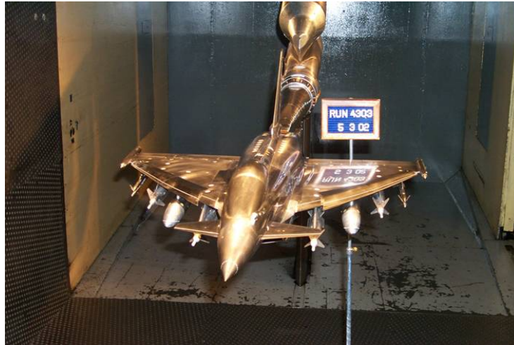
Abb. 2-11: Eurofighter-Modell (Maßstab 1:15), TWT CALSPAN Buffalo NY, USA
