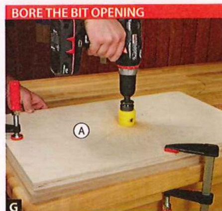
G Clamp the top (A) to a worksurface with a scrap backer board underneath to prevent tear-out. Then drill the bit-access hole.
