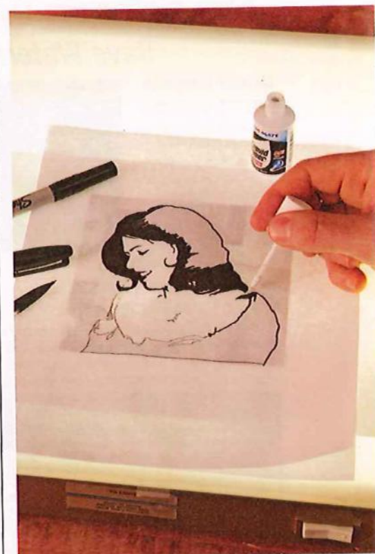
An inexpensive light box makes it easy to convert a high-contrast photo into a black-and-white scrollsaw pattern.
