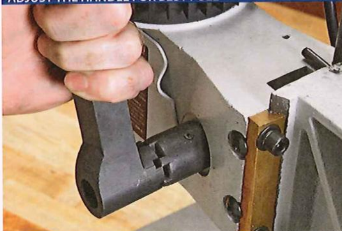
Multiposition handle hubs let you set the most comfortable starting point for the plunge, increasing your leverage and decreasing arm fatigue.
