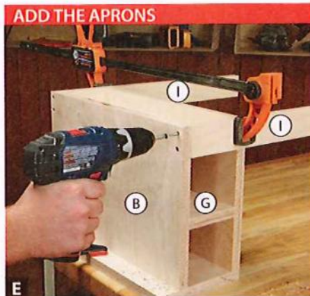
E Glue, then clamp, the table aprons (I) into the notches and flush with the upper divider (F). Then glue and screw the left leg (B) in place.
