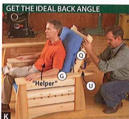
K With the back at the desired angle, clamp the back supports (U) in place. Tilt the back forward to provide room for drilling.
