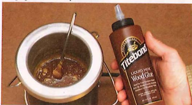
Some modern hide glues, such as Titebond's liquid hide glue, right, are made out of synthetic ingredients. To meet kosher standards, avoid traditional hide glues, left, made from animal by-products.
