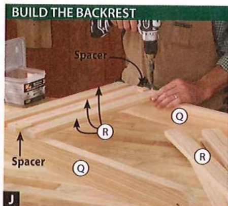
J Position the first rail (R) 1½" from the top of the stiles (Q). Work your way down, using 1" spacers to position the remaining rails.
