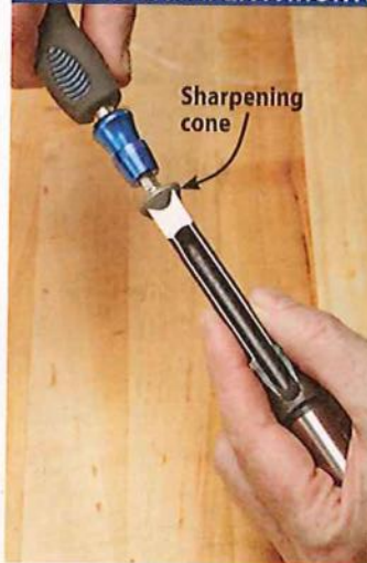
Step 1: Spin the diamond cone tool to hone the inside hollow point of the chisel. Follow up with a finer-grit cone for best results.
