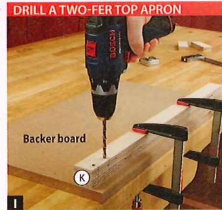
I To ensure that the holes match, stack and secure the top aprons (K) to your bench, with a scrap backer board underneath.
