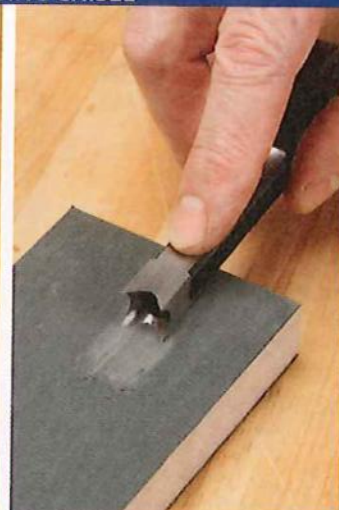
Step 2: After honing the inside, remove the burr on the outside of the chisel by rubbing it lightly a few strokes on 800-grit sandpaper.
