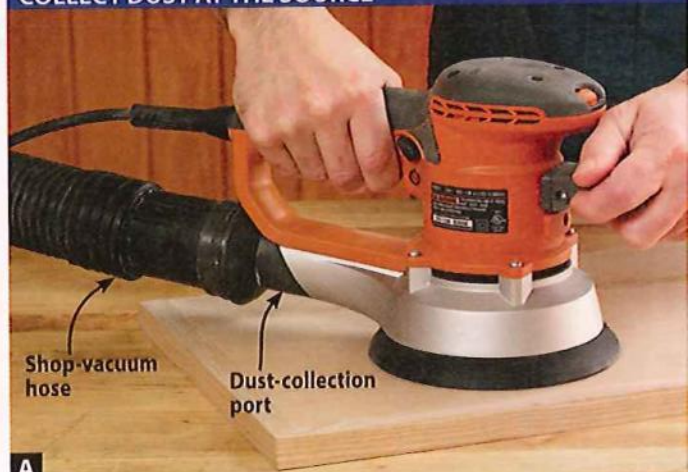
A Tools with dust-collection ports make it easy to capture dust before it scatters across the shop or becomes airborne.
