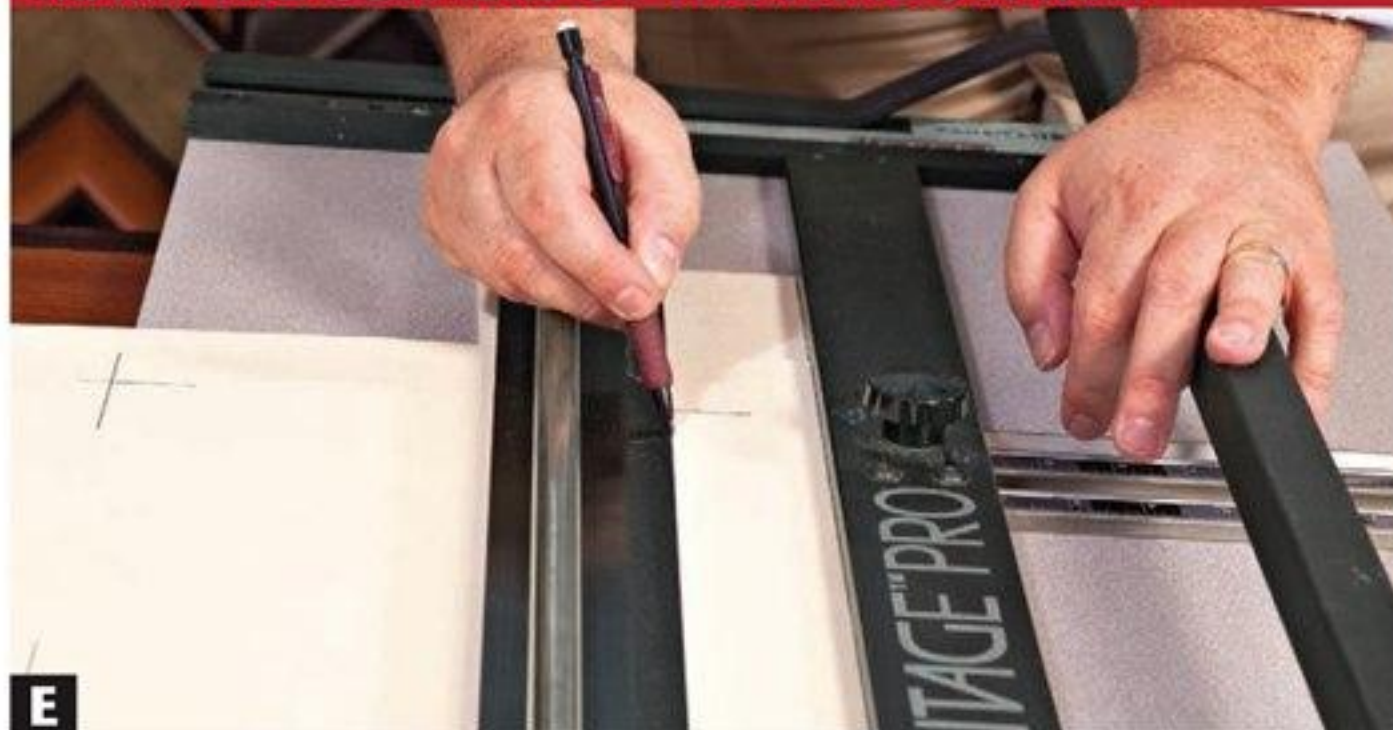
E Using a sharp pencil, lay out crosshairs at each corner to indicate the corners of the window opening.
