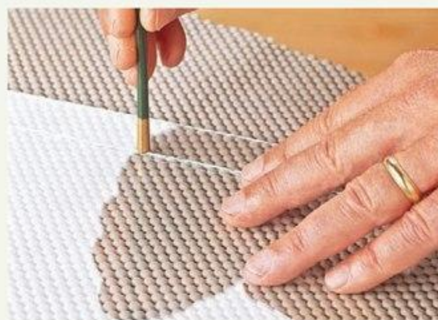
Turn the glass over and with the cutter handle down, use it to tap edge to edge on the visible score line. The glass will separate cleanly as you move along.
