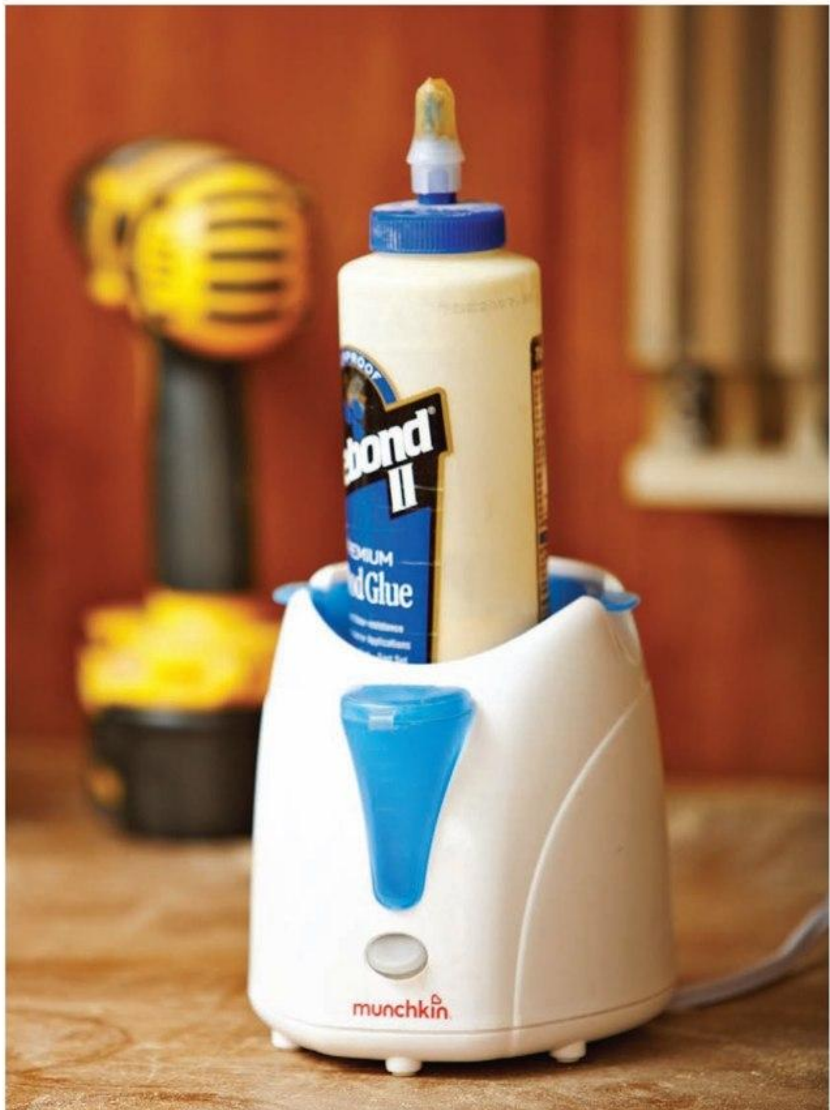
Once you've warmed your cold winter shop, a baby-bottle warmer speeds the process of warming chilled glue.
