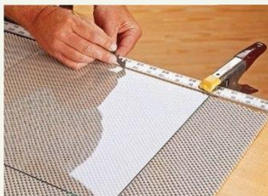
Clamp a straightedge to the glass and brush on mineral spirits. To make a score line, draw the cutter firmly and steadily from one end to the other.
