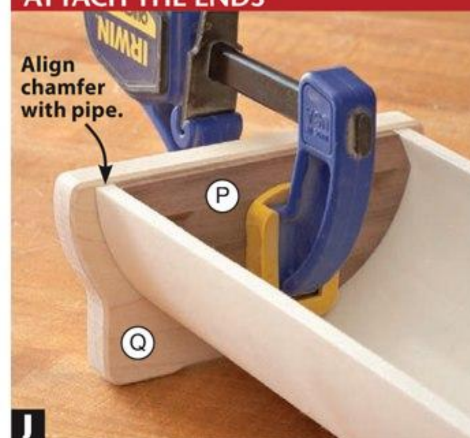
J Glue the ends (Q) to the end fillers (P). Go lightly on the glue to avoid squeeze-out in the cutouts of the ends.
