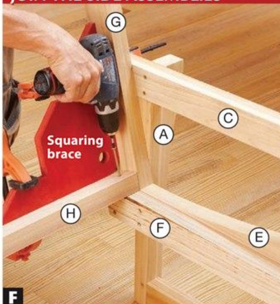
F With a squaring brace clamped to the pieces, drive a 2½" deck screw through the back rail (H) into the end-rail brace (F).
