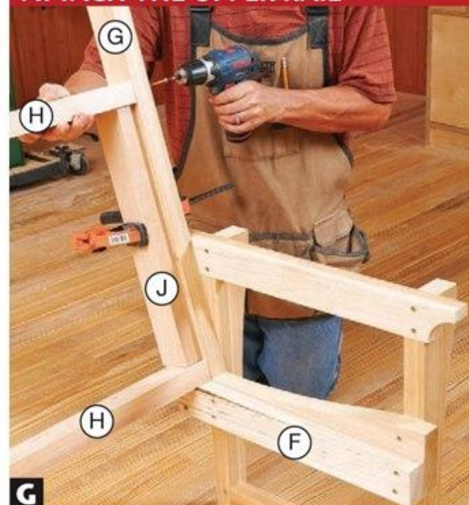
G Position a lower splat filler (J) at each end between the back rails (H), then drive 3" deck screws to secure the upper back rail.
