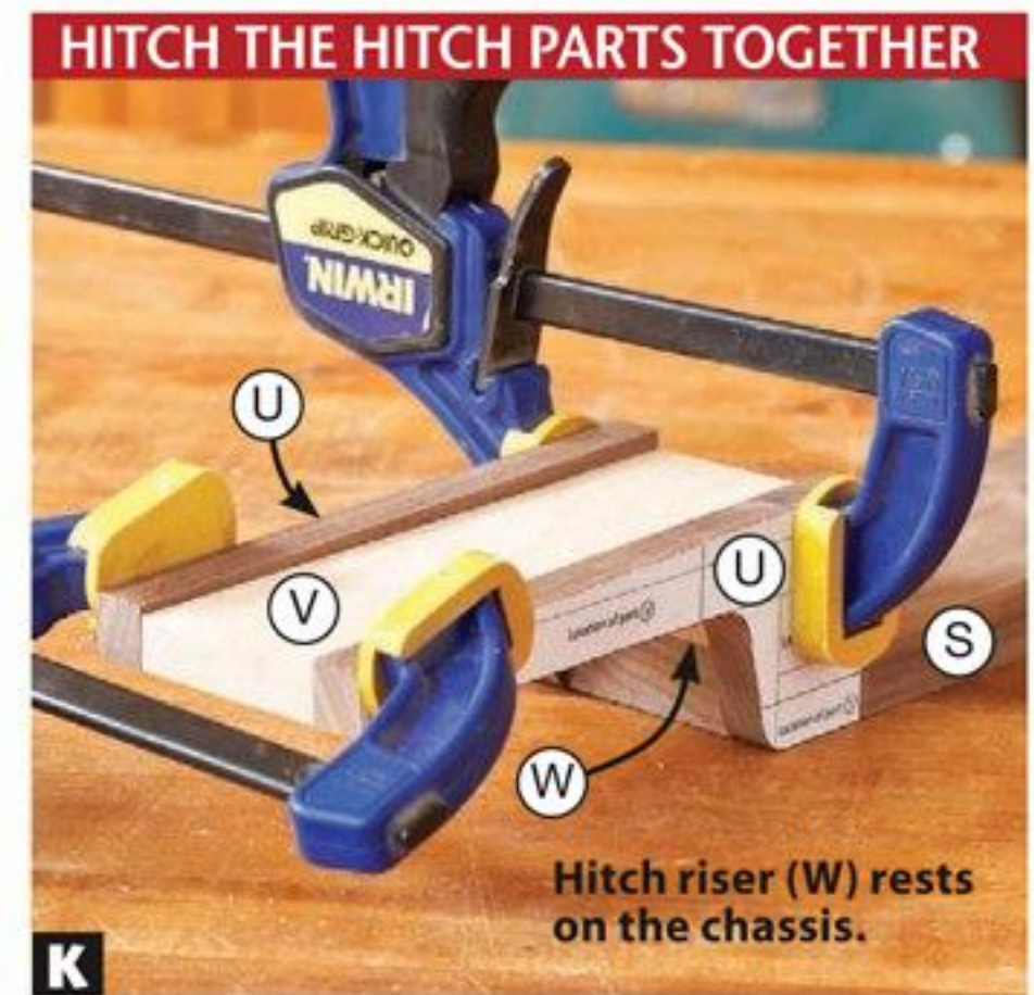
K The chassis (S) helps position the hitch deck (V) and hitch sides (U) during glue-up. Keep the bottom edges and front ends flush.
