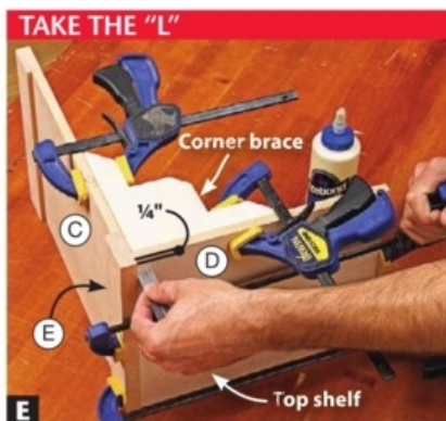
Glue up two L-shaped assemblies. Note that the two assemblies will not be identical. Refer to Drawing 1 and Photo F.
