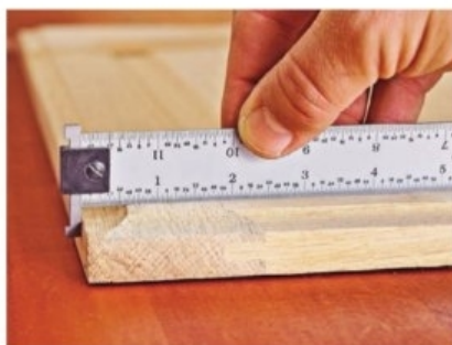
Make sure your tape or rule sits flush with the edge when measuring. This hook rule proves more accurate than a tape's sliding hook.
