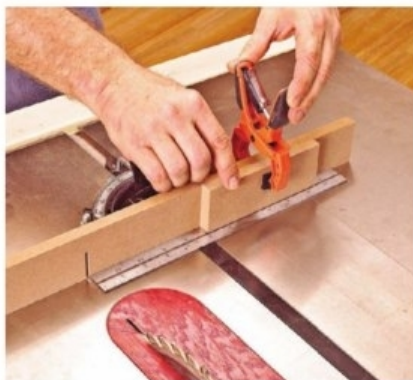
Set a stopblock accurately by measuring from a kerf cut through the miter-gauge extension to the block.
