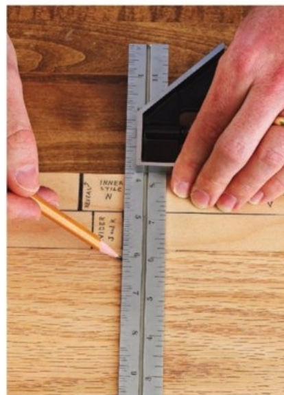
Transfer measurements directly to the part blank, aligning it to display the most pleasing grain pattern or for efficient material use.
