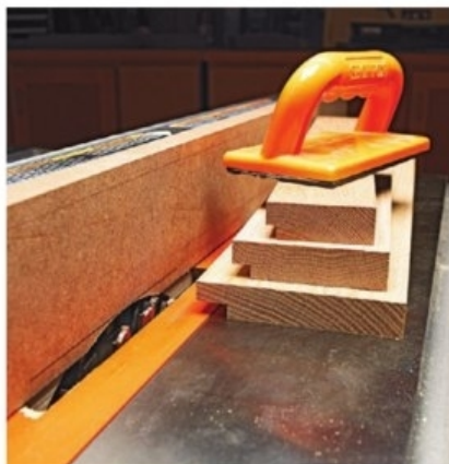
Once you've set up a housed dado stack on your tablesaw, you can cut a variety of rabbet widths by simply moving the fence.
