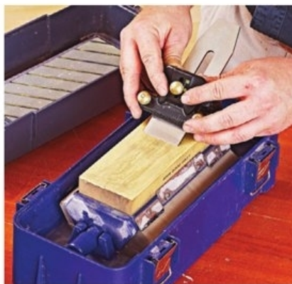
You can sharpen chisels and plane irons on a wheel (left) or flat stone (right). Always use a guide to maintain the correct bevel. Sharpening on a wheel results in a hollow-ground blade.
