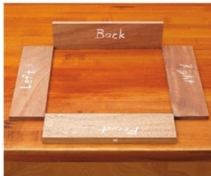
Label parts for position and orientation as you make them. Chalk-marks, shown here, wipe off easily and don't mar the surface.
