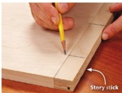
Instead of laying out repeat measurements, lay them out once on a template or story stick for accurate transfer to the parts.
