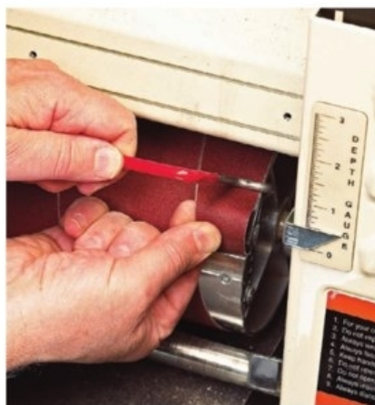
Because the belt clips on both Jet units are difficult to access, use the provided tool to hold the clip open while you insert the belt.
