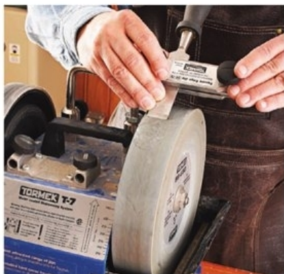
You can sharpen chisels and plane irons on a wheel (left) or flat stone (right). Always use a guide to maintain the correct bevel. Sharpening on a wheel results in a hollow-ground blade.
