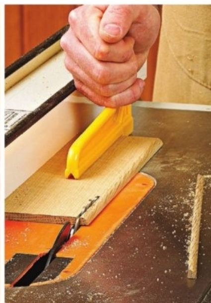
After setting the fence, remove the miter gauge and stop block for each cut. Rout, reset, rip, and repeat as needed.
