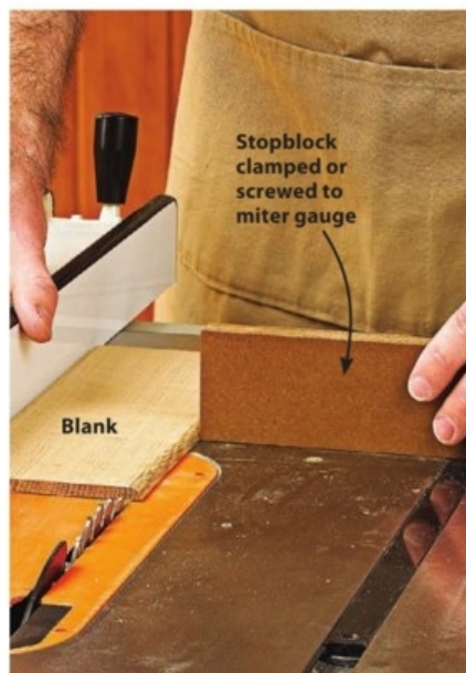
A stopblock on your miter gauge makes it easy to position the fence for repeatable and accurately sized quarter-round trim.
