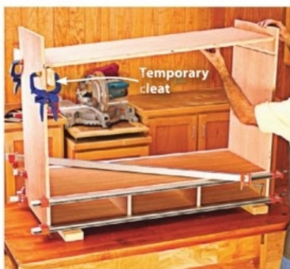
Dry-assembly before gluing this project revealed the need for a temporary cleat to support one end of the shelf.
