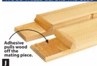
WOOD FAILED BEFORE THE GLUE
