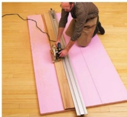
Start with one straight edge on every workpiece. Then rip the opposite edge parallel and square the ends.
