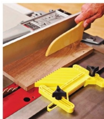
Accessories such as this pushstick and feather board contribute to accuracy and efficiency, as well as safety.
