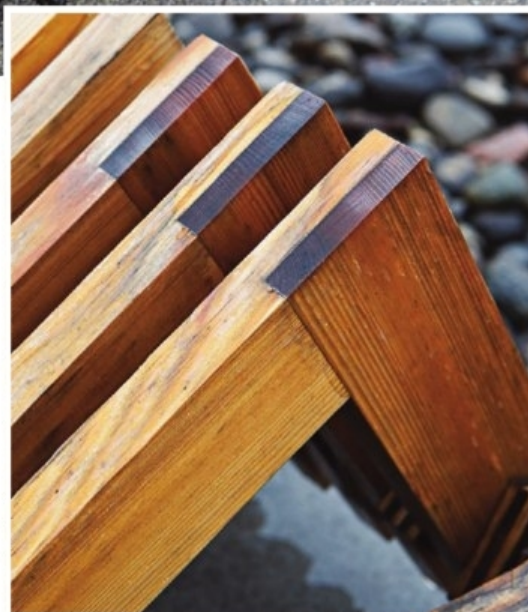
Glue lines on these half-laps wrap around the corner of the samples, while end grain absorbs and wicks away moisture.
