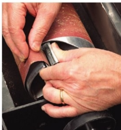
Delta's drum also has spring-loaded clips, but they're easier to access than the Jet sanders' because you can get more fingers on them.
