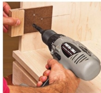
A simple template saves layout time and ensures accuracy for such jobs as drilling screw holes for hardware.
