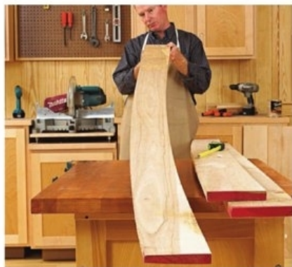
This board obviously needs work before it's ready to use. Cutting it into shorter lengths minimizes waste. Square all stock.
