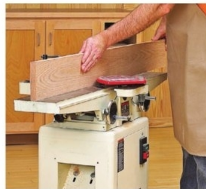
Jointing is essential for stock preparation. A router fills the bill if you don't have a jointer (see Resource 3 on page 69).
