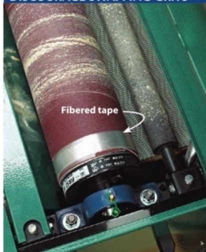
To keep the Grizzly and Shop Fox sanding belts from coming loose and flapping, wrap each end with fibered tape or duct tape.
