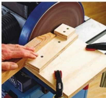
This shop-made jig sets both the angle and length for sanding matching leg bevels, enabling quick and accurate work.
