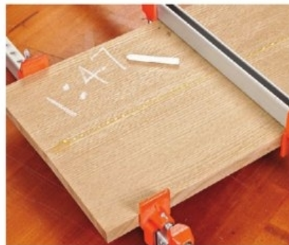
When you glue up several panels, mark each with the time you clamp it so you can keep track of the curing time.
