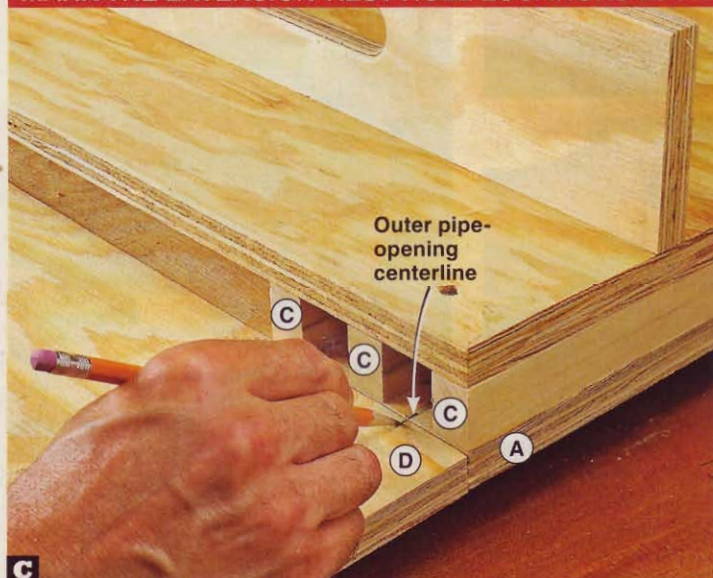
C With the ends of an extension rest (D) aligned with the bottom platform (A), extend the centerlines from the pipe openings.
