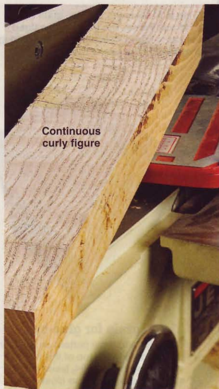
Just one pass on the jointer exposes curly grain that adds character to a project.
