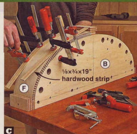
C Using hardwood strips to distribute clamp pressure and working from the center to the ends, clamp the aprons (F) in place.
