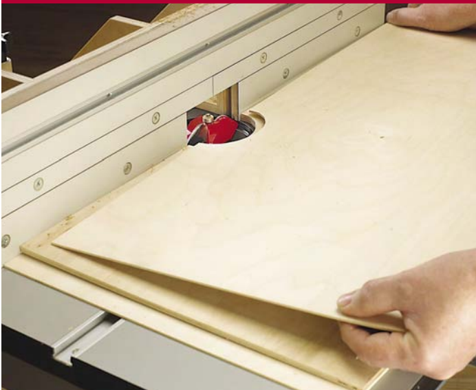
Stack the 1/8" thick spacers on the router table top and secure them with double-faced tape.
