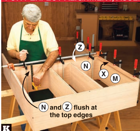
K Glue, biscuit, and clamp the lower rail (Z) in place, keeping the top edge of the rail flush with the top face of the bottom (N).
