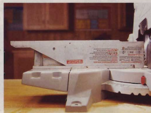
For solid support of 0° bevel cuts, Milwaukee's left fence can be oriented as shown above , or flipped for bevel cuts.
