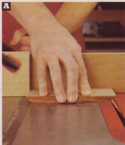
A Use a stopblock to ensure consistent positioning of the spline grooves in the mitered ends of the box parts.
