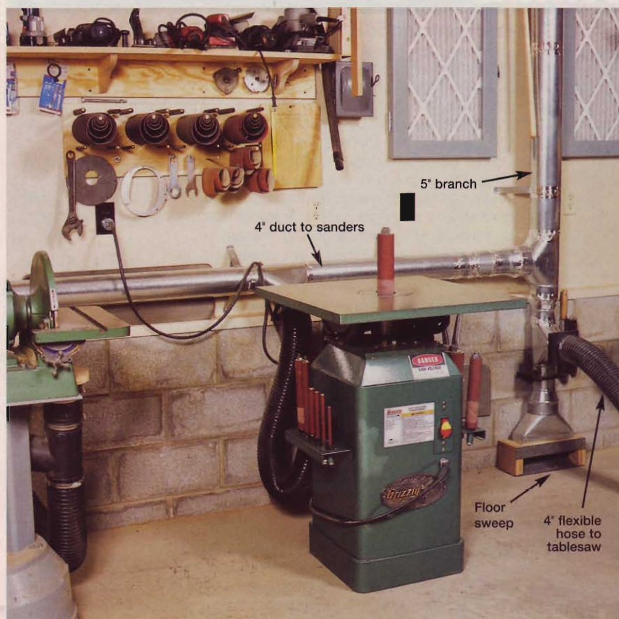
Sharing duties reduces duct length. Here, one 5" branch serves the tablesaw, floor sweep, and a 4" pipe to two sanders. Blast gates direct airflow to just the ports in use.
