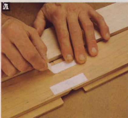
Align the sides (A) with a straightedge, slipping the glass stop (B) underneath so the sides lay flat. With the points of the miters touching, apply masking tape.
