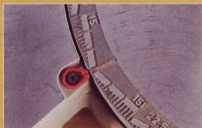
GOOD: Despite a small gap between it and the cast-in scale, Ridgid’s fine-line cursor reads easily and accurately.
