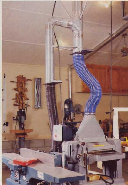
To reduce the number of long duct runs, a 5" section does double duty, serving the 15" planer and a 4" branch to the jointer.
