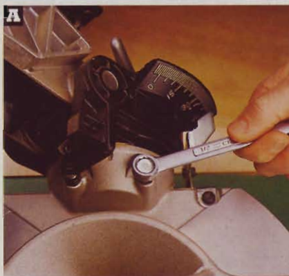
A Different miter saws have different methods of adjustment, but this is a common situation. The saw head rests on a bolt when set for vertical cuts. Turn the bolt to adjust the setting to exactly 90°.
