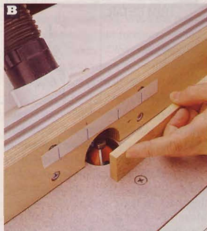
Use the inner set of start/stop lines on your router fence when routing the stopped chamfers on the horizontal trim, and use the outer lines when routing the vertical trim.
