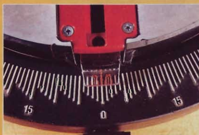
FAIR: Pro-Tech offers a hairline cursor and vernier scale, but the dark background makes it difficult to read.
