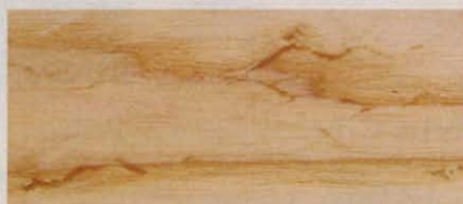
These zigzag tracks are remnants of tunnels made by the cambium miner, a larvae that feeds on the new-growth layer (cambium) under the bark. After the larvae leave, new growth fills the voids.
