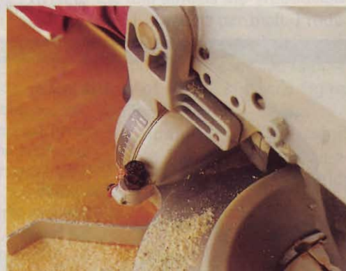
Makita's bevel-scale cursor hides behind the knuckle and 45° stop. Reading the scale becomes harder yet as you tilt the head to bevel.
