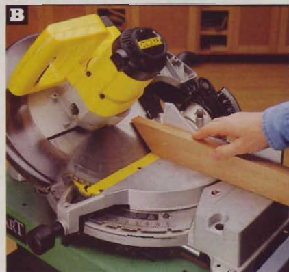
B Use the 45° angle setting to cut a template for the 45° bevel setting. It's easier to slide a piece of wood against the blade than to fit a combination square under the opposite side.
