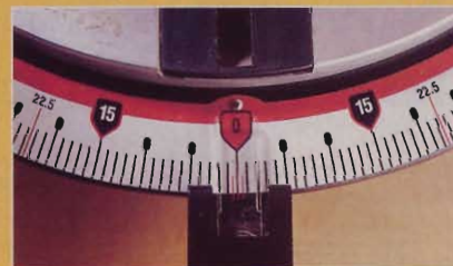
EXCELLENT: A hairline cursor, vernier scale, and high-contrast background place Black & Decker’s miter scale among the best in the test.
