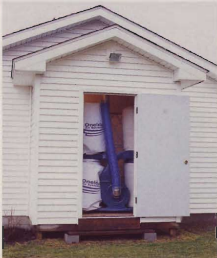
A shed houses the dust collector outside the shop. The large bags on the left are oversize, 1-micron units; at right, the collector's stock 20-micron bags.
