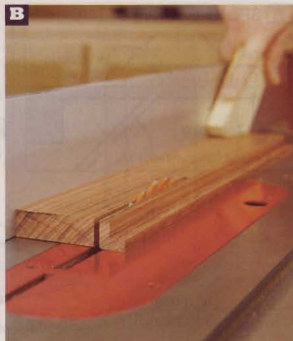
B With the rabbet facing up, rip a \frac{3}{4} "-wide strip from the blank. This rabbeted blank will form the feet (F).
