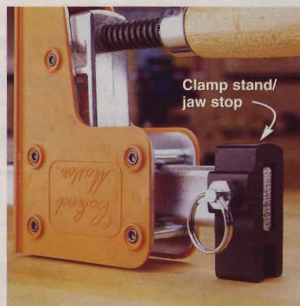
Cabinet Master's clamp stand/jaw stop raises the bar so the jaw slides smoothly. The stop removes easily to convert the clamp to a spreader.
