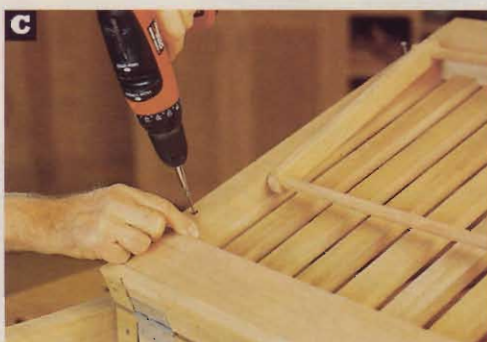
C After placing the brackets (P) and dowel/brace assembly (N/O) in the back platform, drive in the mounting screws
