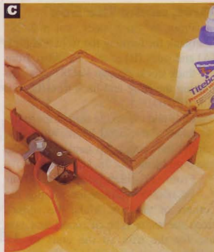
C With the box on a 1" spacer, make sure that all four feet touch the work surface before tightening the band clamp.
