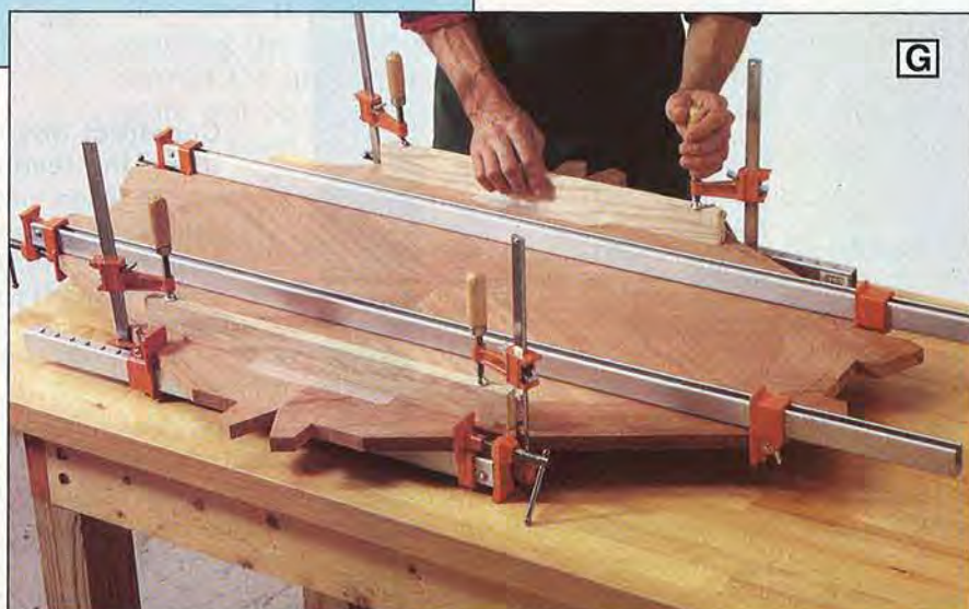
After joining the field quarters into halves, glue and clamp the halves together. Trim band waste when the glue dries. Profile the edge of the top with a router or leave plain. Then, finish-sand and apply a clear finish.
