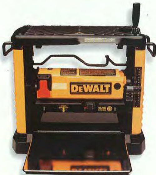
The DW733 12 1/2" Portable Thickness Planer features a four-column head lock which stabilizes your work, greatly reducing snipe.
