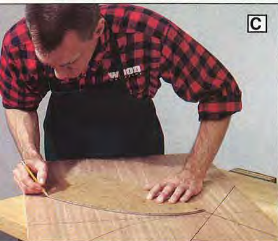
With the master template, lay out the top on the mahogany plywood. Here, we laid out the top in a sunburst pattern.
