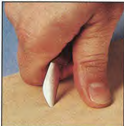
You'll hold the knife this way for most cutting. Keeping the end of the thumb and the index-finger knuckle on the workpiece maintains the proper angle.
