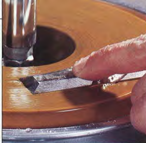
To lap a chisel, place the back side on the wet wheel with the wheel spinning away from the cutting edge as shown.
