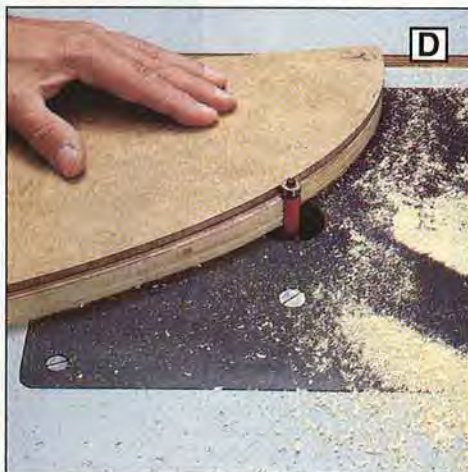
After sawing out the field sections with a jigsaw, true the curved edges with a flush-trimming bit at the router table.
