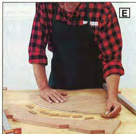
Space and dry-fit single 2"-long splines of \frac{1}{8} " tempered hardboard into the slots of the field/band joints.
