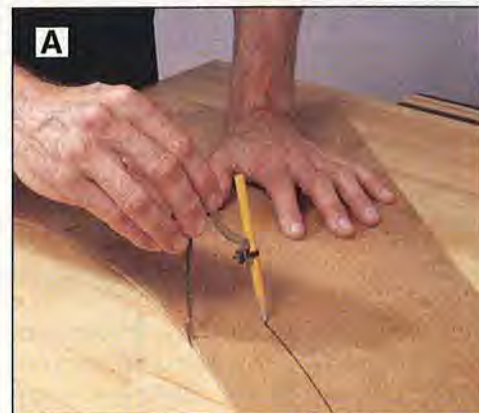
Mark the band-section template stock with a compass set to 2". Draw the line to parallel the curve of the field.
