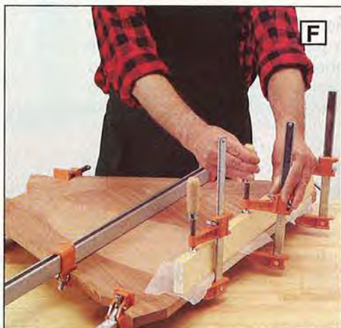
Notches in the band-section blanks allow a tight glue-up to the field quarters. A glue block keeps the pieces flat.
