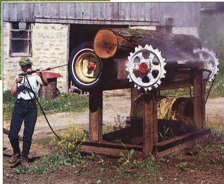
Cindy Huppert, Jim Birkemeier's partner, pressure-washes a log of red oak to remove dirt that would otherwise dull the mill's bandsaw blade. The homebuilt rack slowly turns the log via an electric chain-drive mechanism.
