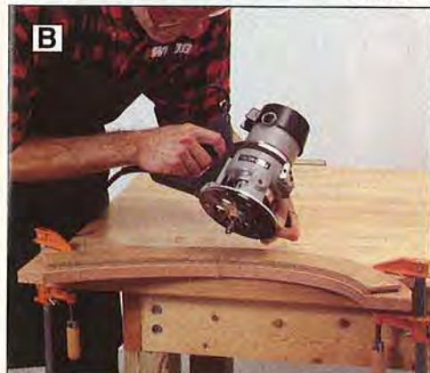
To match the band-section template, trim away \frac{1}{8} " from the band-section stock with a handheld router.
