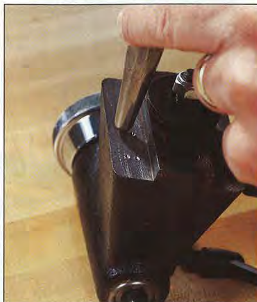
Punch marks raise small rings of metal around the depression, raising the tailstock slightly. Sliding will wear the rings down after a while.
