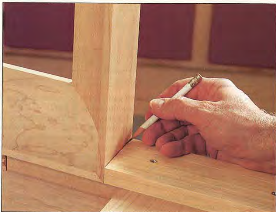
Mark the length of the shortest piece of cove molding onto the cove molding stock as shown. Cut this piece and clamp it as shown on the next page.
