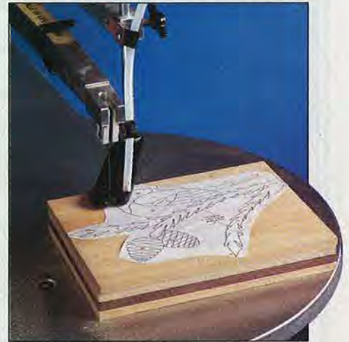
Adhere the full-sized paper pattern to the top of the stacked lamination, and scroll-saw the pieces to shape.
