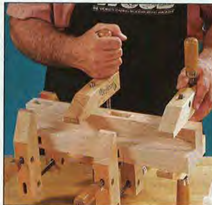
Use handscrew clamps to hold the splined leg pieces together at a right angle until the glue dries.
