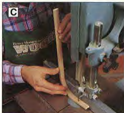
C Using a bandsaw fitted with a \frac{1}{4} " regular 14-tooth-per-inch blade, rip the runner lamination down the center.
