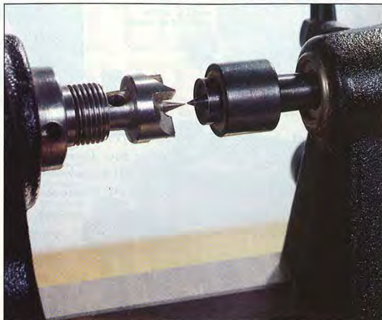
When the points on the centers meet exactly and run on the same axis, you'll be able to turn a cylinder accurately on the lathe.
