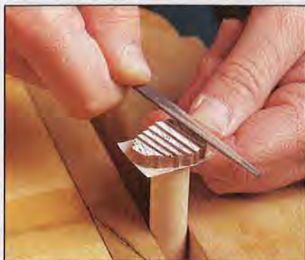
A 4"-long piece of \frac{5}{8} " dowel stock makes a sturdy handle for filing and sanding the pine cones to shape.
