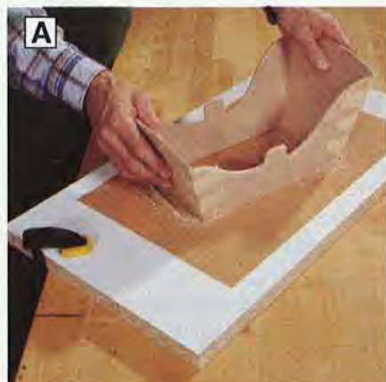
A Use sandpaper adhered to a smooth flat surface to sand the bottom of the sleigh body flat.
