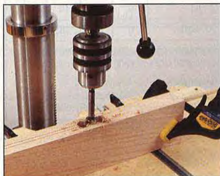
Remove most of the waste from the marked mortises with a Forstner bit, using a fence and stops on your drill-press table for alignment.
