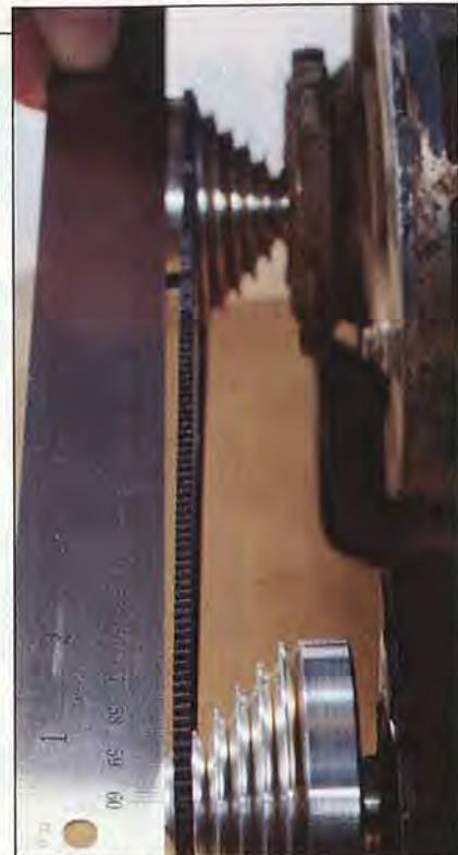
The belt should run parallel to the pulley grooves. In this case, the motor pulley (top) should be moved outward (to the left) on the shaft.
