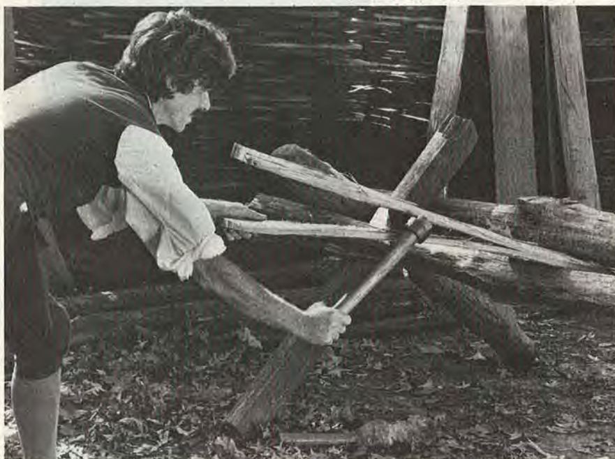
The froe gives you the strength of ten for the final splitting. The forked limb gives you the leverage to keep the split running true.
