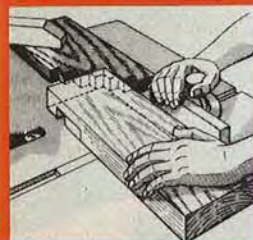
Use a notched stop block to control the width of cut for a lap joint.
