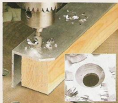
▲ Metal Work. Smooth countersinks in soft metal, like brass or the aluminum shown above, are a snap with a Weldon countersink.
