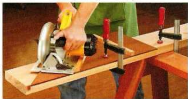
▲ 45° Miters. To make precision 45° miters, align the angled end of the crosscut guide with the layout mark. Then run the base of the saw against the fence as you make a cut.
