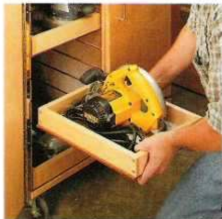
A. Adjustable Height. If your storage needs change, just slide a tray out and then slip it back in at a different height.
