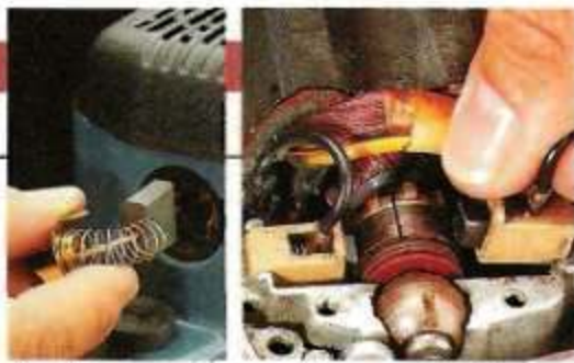
Brush Access – A removable cap makes it easy to take out some brushes (left). The only way to remove other brushes is to open the case (right).
