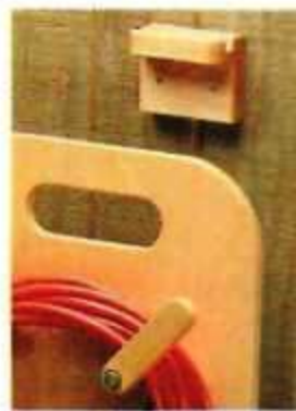
▲ To hold a single caddy, an L-shaped wood block with a groove in the top provides a handy, wall-mounted hanger.
