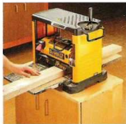
C. Tool Stand. With a sturdy top and a set of locking casters, this cart can also serve as a stable platform for a benchtop tool.
