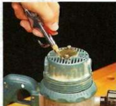
A. Remove Dust – With the tool running, blow air through the intake slots to remove packed-in dust.
