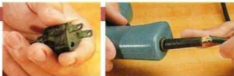
▲ Check for Damage. To avoid the possibility of a serious electrical shock, replace a plug if it's missing the grounding prong (shown at left) or a power cord with a break in the outer sheath (right).
