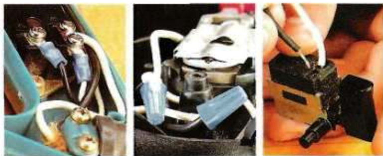
▲ Connectors. The wires from the power cord may be attached with crimp-on connectors (left), wire nuts (center), or a spring-loaded mechanism in the switch (right). Just be sure they're tight so they don't wiggle loose.
