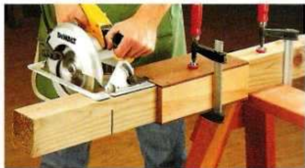
▲ Cutoff Saddle. To ensure smooth, square cuts when working with thick lumber, this cutoff saddle guides the saw when making cuts from two opposite sides of the post.
